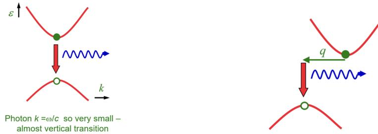
Indirect bandgap material (e.g. silicon): states are displaced in k-space and so addition of momentum from a phonon is required to effect a transition from one band to the other. Light emission much less likely and a lot of energy dissipated as heat.
