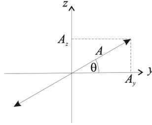
Figure 1: Linear polarisation
