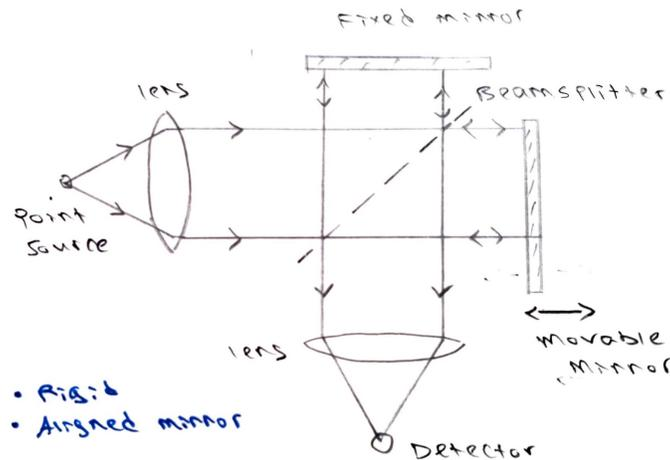
1. How it works: light from a point source is transformed into parallel beams and then split at the beam splitter. They travel along different perpendicular paths and finally recombine and focused at the detector.
