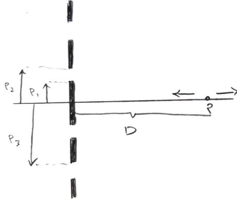
Figure 4: D is the focal length
